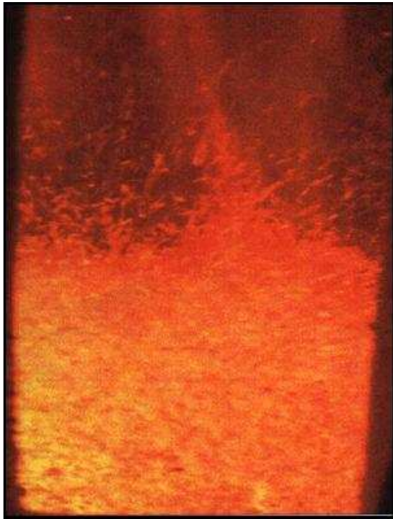
Fig. 18 A photo for fluidized bed using coal m_{LPG} = 0.3121 g/s, m_{Coal} = 1.092 g/s, m_a = 41.1 g/s. Bed material: sand
