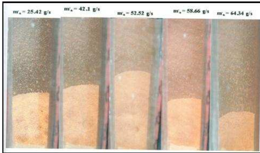
Fig. 6 Limestone cold tests
