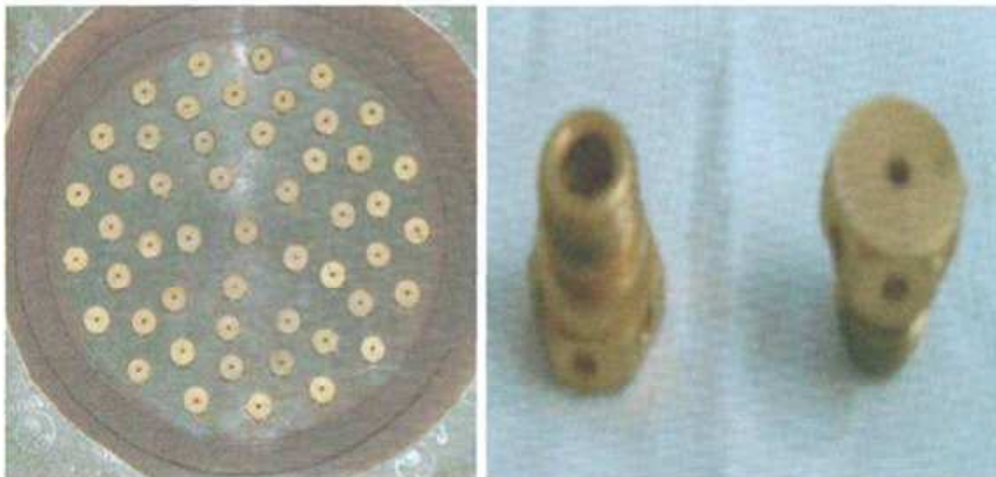
Fig. 2 Distributor plate and nozzles
