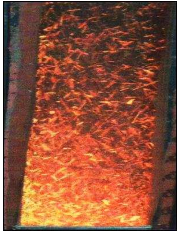
Fig. 19 A photo for fluidized bed using wood chips m_{LPG} = 0.3121 g/s, m_{wood\ chips} = 1.092 g/s, m_a = 41.1 g/s Bed material: sand
