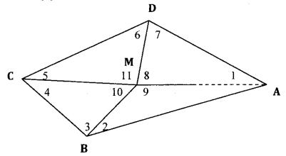
ABCDM is a is a part of a free triangulation network chose angles 1 to 11 as the following figure. Calculate the condition equations for its adjustment and write them?
