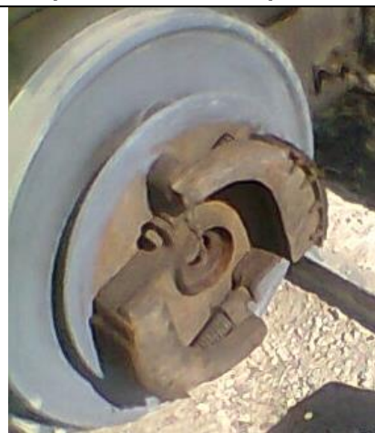
Fig. (1) Assembled shoes on disc fixed upon engine flywheel.
