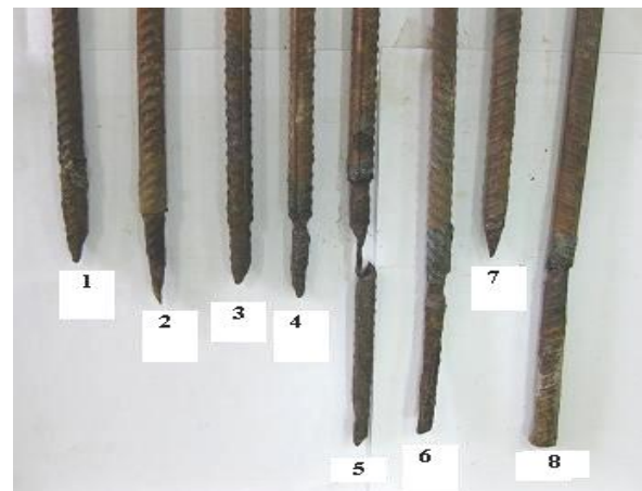
Fig. 13: Corroded steel bars due to chloride attack at the end of the test (1; C0W, 2; C0LW, 3; C10W, 4; C10LW, 5; C20W, 6; C20LW, 7; C30W, 8; C30LW)
